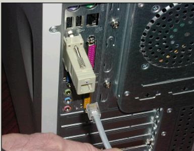
Attach one end of the telephone-like cord into the hooded connector.
